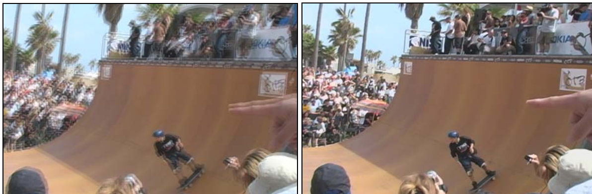
Double imaging on interlaced material is a typical problem with poor quality systems. Compare the standard processes on the left with AmberFin on the right. AmberFin produces clean results.
